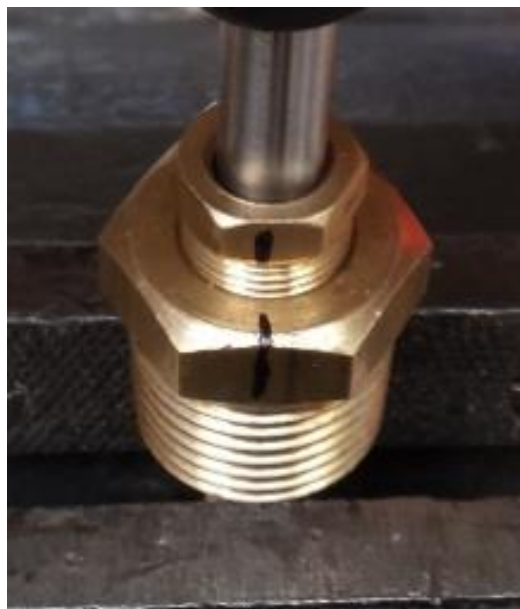
Figure 3-3. EXAMPLE PEN MARKS TO ENSURE CORRECT ROTATION IS APPLIED.
