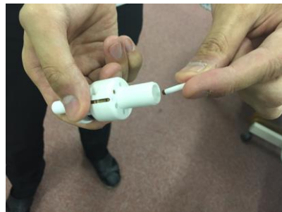
Introducing rotor in rotorcarrier
