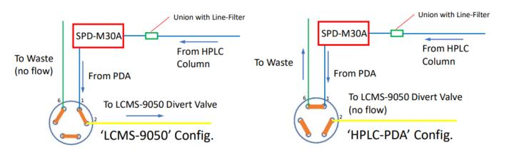
Note that the Left-hand Configuration and Valve Position would now remain the same when using the SPD-M30A and LCMS-9050, in Tandem.
