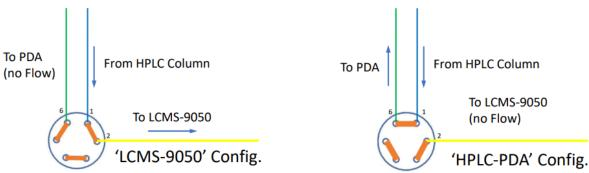
Connect outlet from HPLC column to *Port 1*, on the valve (inlet *from* HPLC column). Select *Switching-Valve Position* '1' in the software (currently the Default for LCMS-9050 Configuration) Apply flow to column, and determine from which port ('2', or '6') solvent flows
