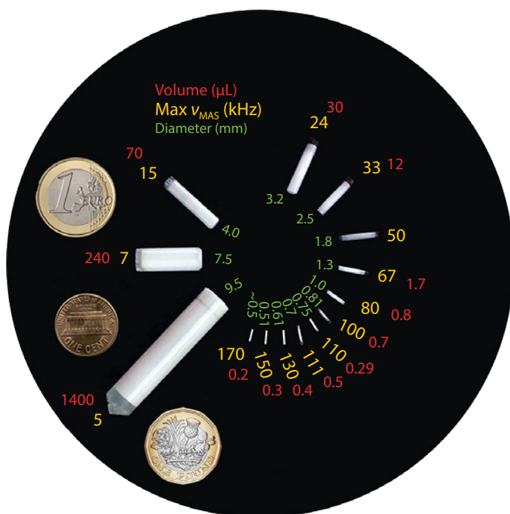
Fig. 14.3: The rotors with different outer diameters used for measuring solid-state NMR spectra. The image shows the sample volume (in \mu L , red numbers), the maximum magic-angle spinning speed (in kHz, orange numbers), and the outer rotor diameter (in mm, green numbers). Some common coins are included for comparison. The picture has been provided by Prof. J. Lewandowski (University of Warwick)
