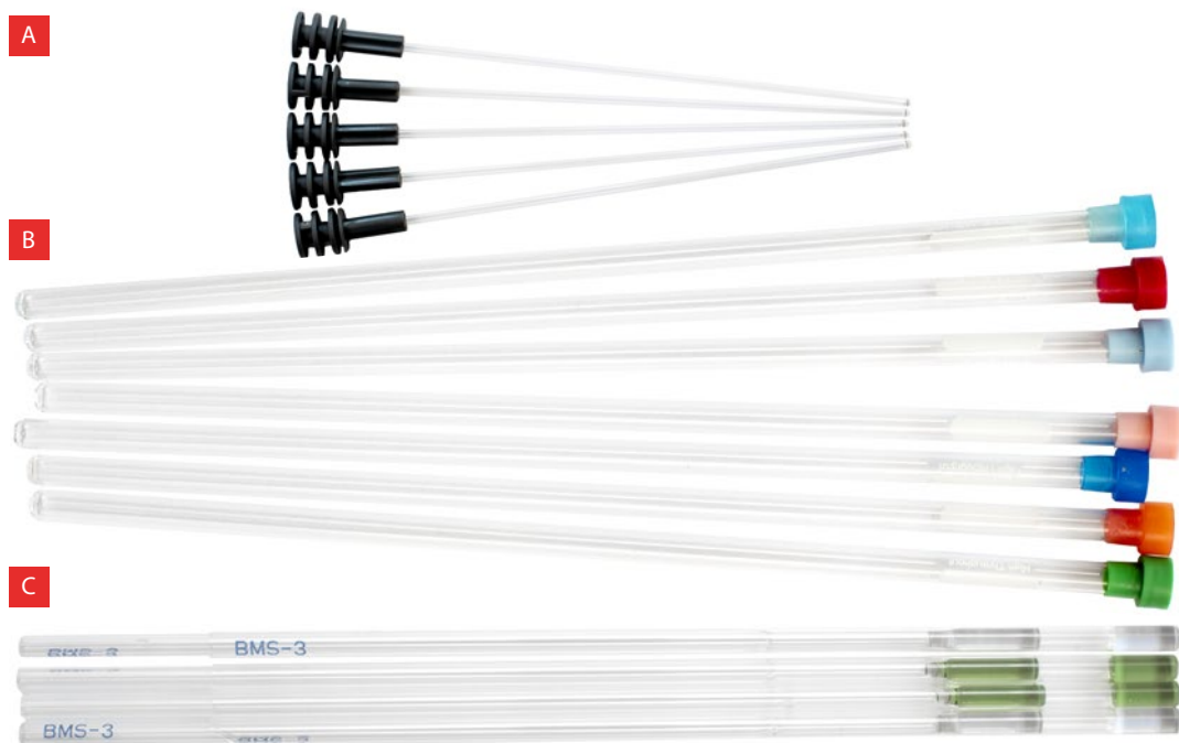
Fig. 10.3: NMR tubes: micro (A), standard (B), Shigemi (C)
